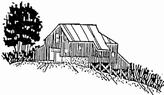
Inappropriate Foundation Treatment
